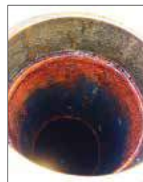
Figure C: Rusty Tank Filler
